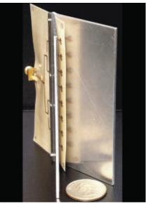
▲ Fig. 9 Photograph of the fabricated antenna array with corner reflector.
