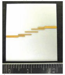
▲ Fig. 5 Photograph of the 10 GHz parallel-coupled line filter using DPC technology.
