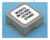
Modco announces its MCS Series CRO's. Low Vcc of 3.3V and current consumption of 13ma and makes it ideal for battery powered applications. Model Number MCS1400-1470CR tunes 1400-1470MHz with a Vt of 0.3-2.7V It provides 0dBm output power. Phase Noise is -110dBc @ 10kHz Pushing is 0.2MHz per volt and Pulling is 0.9MHz. Many models are available. www.modcoinc.com
