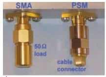
$\blacktriangle$  Fig. 2 Connectors shown from the side mated with a 50  $\Omega$  termination (SMA) and a cable connector for the EZ141 cable (PSM).
