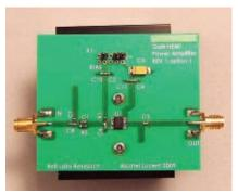
Fig. 5 Test board of broadband GaN HEMT power amplifier.
